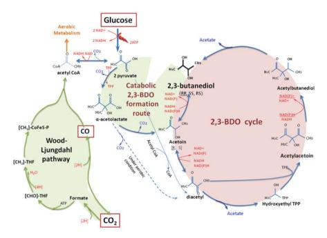
**Fig. 2** Different pathways involved in the formation of 2,3-BDO in bacteria (after [5, 35]). *THF* tetrahydrofolate
