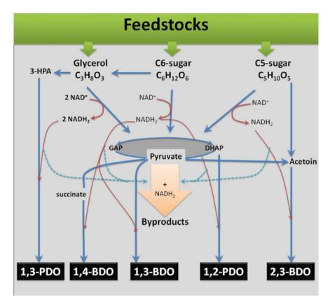
Fig. 1 Major routes for bioproduction of diols from different feedstocks (modified after [2]). 3-HPA 3-hydroxypropionaldehyde, GAP glyceraldehyde 3-phosphate, DHAP dihydroxyacetone phosphate
