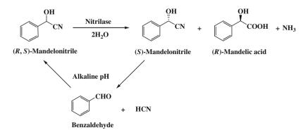
Fig. 17 Nitrilase-catalyzed synthesis of (R)-mandelic acid from racemic mandelonitrile in a dynamic kinetic resolution manner
