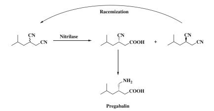
Fig. 26 Nitrilase-catalyzed synthesis of (3S)-3-cyano-5-methyl hexanoic acid from racemic isobutylsuccinonitrile
